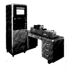
Ultraviolet near infrared spectrophotometer announced by Beckman. First commercially available instrument designed specifically for near infrared region of spectrum is claimed by manufacturer. Using a photomultiplier detector for ultraviolet work, the instrument offers a wave-length range from 220 to 270 m $\mu$
